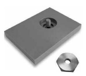
When the sheets are bolted into position with studs and hex nuts, we recommend a nominal distance of 250 mm. The distance between the holes and the edge of the sheet should not exceed 50 mm.
